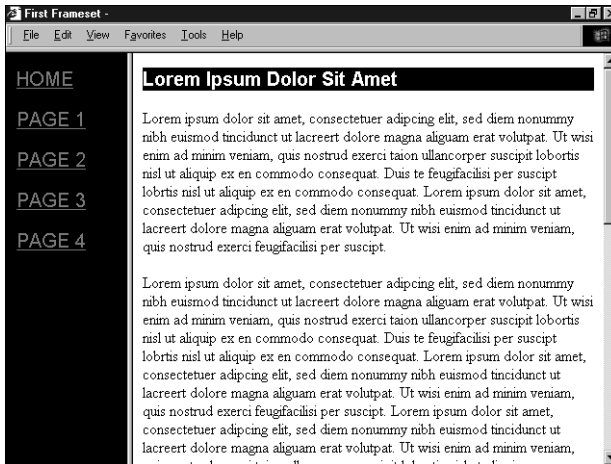
FIGURE 10.1 A simple two-frame document as it appears in the browser. The left frame contains the site's navigation bar and the right frame contains the pages to which the navigation buttons link.
