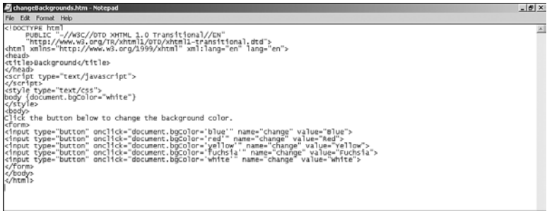
FIGURE 14.2 Simple JavaScript code to change the background color with the onclick command.
